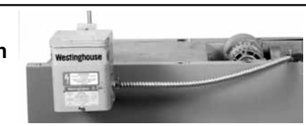
FIGURE 5 - Install Transformer Bracket
